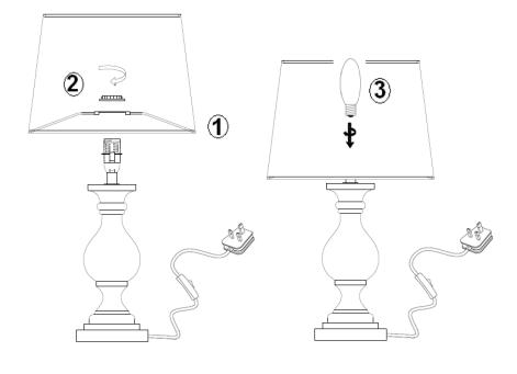
To use this item in Europe, the 3 pin adaptor can be removed by loosening the central screw and removing the adaptor to reveal the 2 pin Europe plug.
